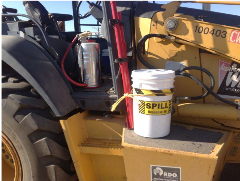
Photo 3: Spill kits are maintained onsite in accordance with MM-HAZ-1A and the Hazardous Materials Management Plan.
